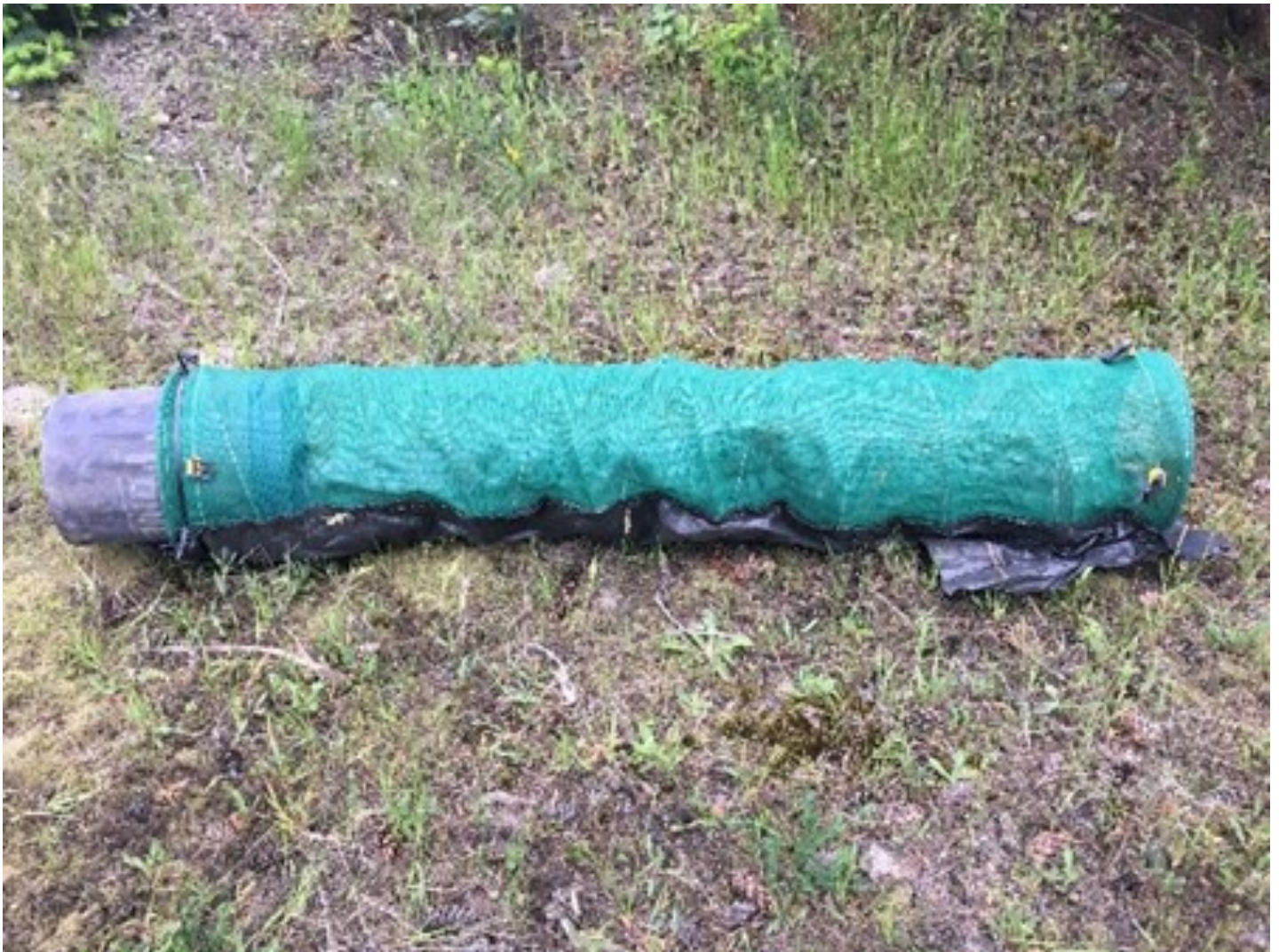
A typical homemade non-compliant fish screen made from a bucket and screen door mesh
